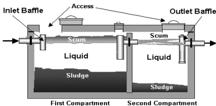
A typical septic tank system normally operates by gravity, and consists of a tank and a soakaway drain. Untreated wastewater from a property flows into the septic tank, where the solids separate from the liquids. Some solids, such as soap scum or fat, will float to the top of the tank to form a scum layer. Heavier solids,
