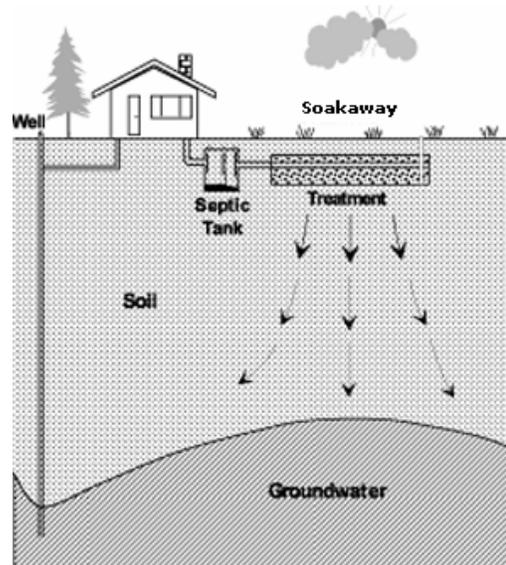
In some areas of the South Africa, the seasonally high water table is within a 600mm of the ground surface. Therefore a soakaway may be typically installed close to the surface of the ground, but care must be exercised as it is possible that the polluted water may break through the ground surface. In other areas there may be clay ground present close to the ground level, and where this occurs then it is very unlikely that the use of a soakaway will prove satisfactory.
